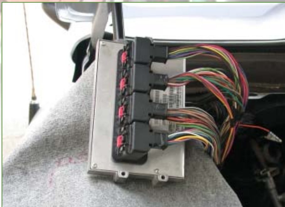
Figure 1: Computer Connectors The PCM wiring harness has four connectors, numbered 1 to 4.
